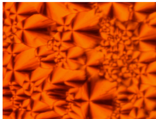
FIG. 9. (Color online) Optical texture of compound III at 163 °C on cooling from the isotropic phase with the sample between two glass slides. The red color is due to the absorption of the compound. Picture is 240 \mu\text{m} wide.
